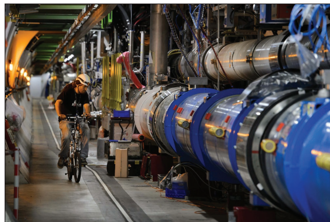
Figure 1.10 The Large Hadron Collider (LHC) is an accelerator used to study interactions of subatomic particles at very high energies. It is located at CERN, the European Particle-physics laboratory in Switzerland. ©Fabrice Coffrini/AFP/Getty Images)
