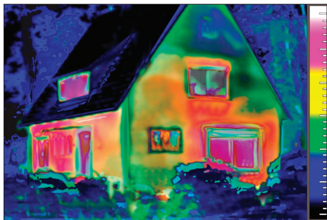
Figure 1.8 An infrared photograph showing patterns of heat loss from a house is an application of thermodynamics. ©Dirk Püschel/Getty Images RF
